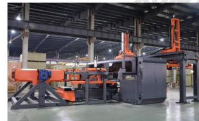
滤板五轴联动加工线 Five-axis processing line for filter plate
