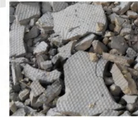
过滤后滤饼含水率45%-60% Moisture content of filter cake 45-60%
